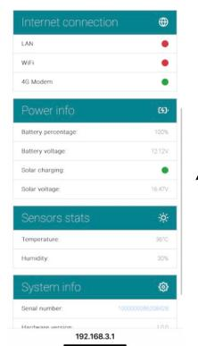
Check solar panel is connected (Log into the system via wifi on your phone and check solar power is working
